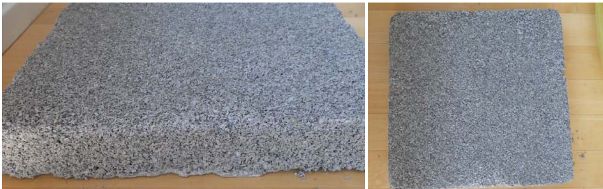
Figure 2 - Screed coat containing NUMIX aggregates
